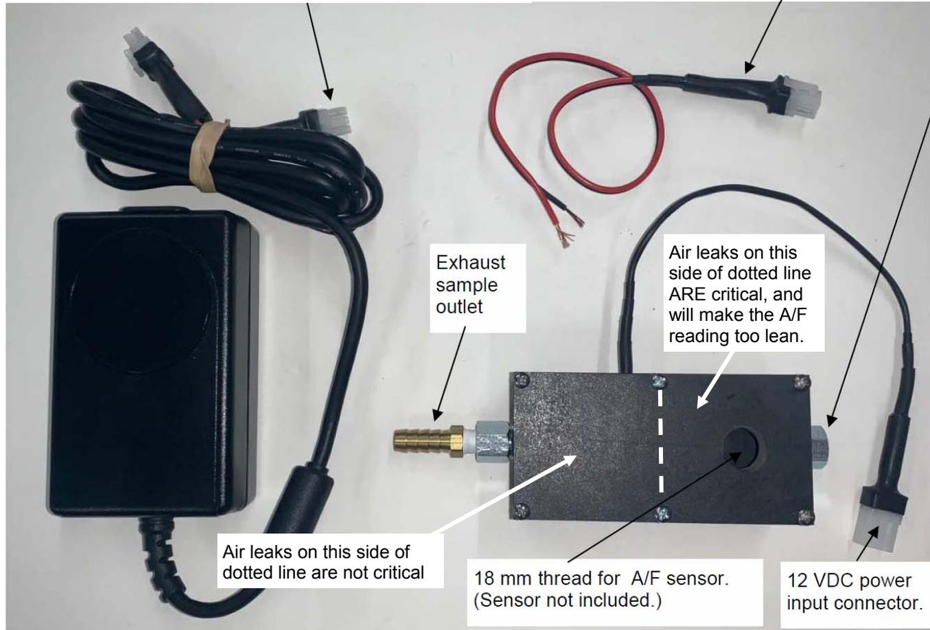
Inlet is fitting closest to A/F (O2, lambda, wideband, etc) sensor. Use 2-3 feet of metal tubing at the enclosure (for cooling the sample), then flexible tubing, and then a metal probe which you place up inside the exhaust outlet for sampling. Typically 1/4" piece of copper or stainless tubing works for a probe. **DO NOT over-tighten the fittings (inlet or outlet) as you could crack the enclosure.**
